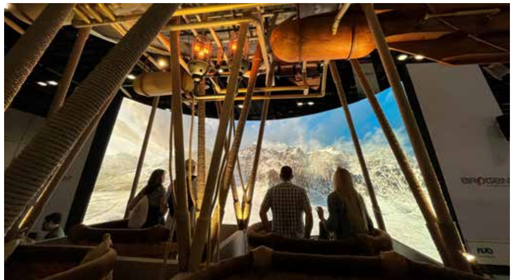
RiseUP combines a motion base platform with a curved LED screen to simulate a hot air balloon ride.
